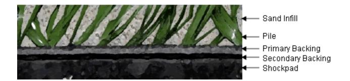
**Yarn**: Polyethylene yarn is preferred as it provides a resilient and durable surface without being too abrasive. A secondary yarn is sometimes used to add strength and stability. Yarn is either monofilament or fibrillated.
